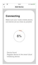
5. In the automatic Network connection mode, indicator flashes Flashes quickly,holds the reset key for 5 seconds with the card Pick-up pin, the indicator flashed slowly, and enters the manual Network connection model. APP chooses compatible model. According to the prompt, enter Wi-Fi password and click confirm. Then switch to the Wi-Fi setting interface, connect smartlife\_xxx Network and return to APP to continue adding devices. Device.
