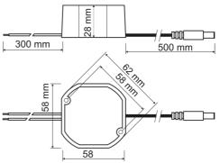
Fig.1. Dimensions of power supply.
