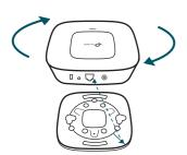
Attach the EAP to the mounting bracket by aligning the arrow mark ▼ on the EAP with the arrow mark ↓ on the mounting bracket, then rotate the EAP until it locks into place, as shown on the left.
